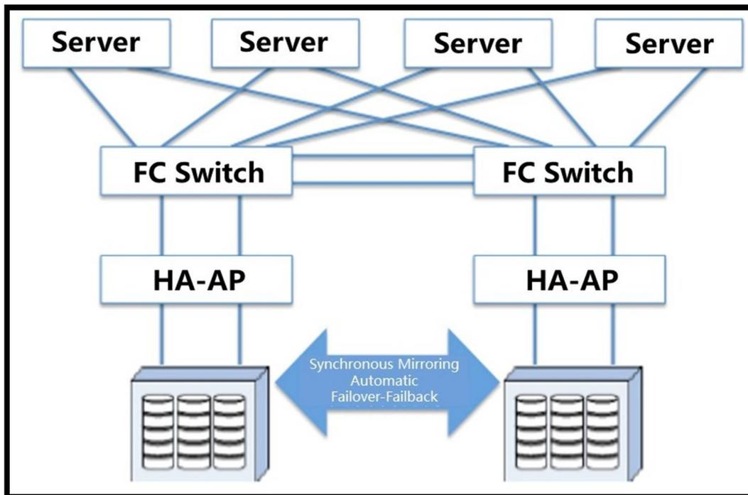
**Figure 3. HA-AP-enabled Active-Active IAAS Datacenter Logical Diagram**
