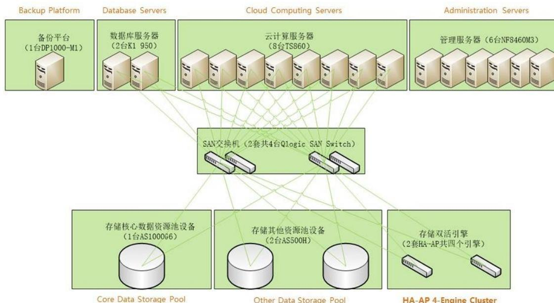
Figure 4. CSSC Cloud-based IAAS Datacenter Topology Diagram
